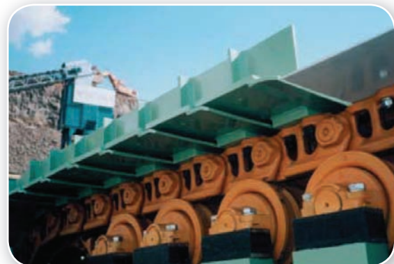
Apron conveyor chains, roller and buckets.
